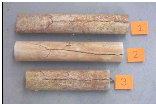
Figure 5 Failed asbestos cement pipe sections
